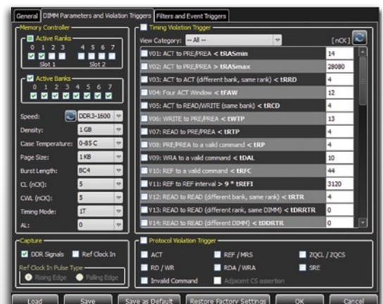
JEDEC timing values load automatically based on memory parameters.
